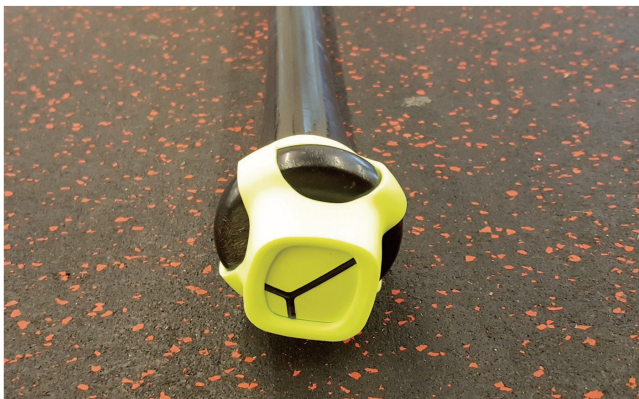
Figure 1 Baseball bat instrumented with the ZEPP sensor.
